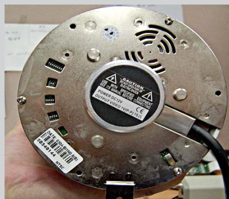
▲ Picture 2: Jumpers at the bottom side of PZT camera base
