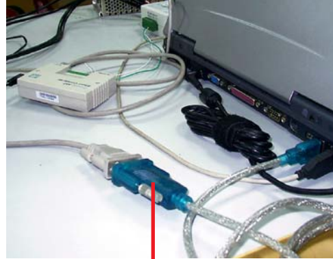
Connect to USB/RS485 converter (DVR without COM Port or for long distance usage)
